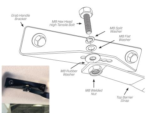
For the other end of the **Top Barrier Strap**. Place **M8 Crinkle Washer**, **M8 Flat Washer** and **M8 Nylon Washer** onto the **25mm MSA Barrier Knob**. Slide through the **Cargo Barrier**. Place the **M8 Rubber Washer** between the **Cargo Barrier** and the **Top Barrier Strap**. Tighten the bolt assemble into the welded nut in to Upper side of the **Top Barrier Strap**. Repeat this process for the other side bracket assembly.
