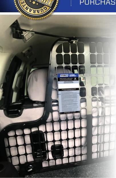
A quality MSA 4X4 Cargo Barrier is easy and safe to install into your vehicle. It utilises the existing holes for the rear grab handles.
