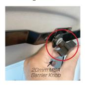
For the other end of the **Top Barrier Strap**. Place **M8 Crinkle Washer**, **M8 Flat Washer** and **M8 Nylon Washer** onto the **25mm MSA Barrier Knob**. Slide through the **Cargo Barrier**. Place the **M8 Rubber Washer** between the **Cargo Barrier** and the **Top Barrier Strap** and tighten. Repeat this process for the other side bracket assembly.
